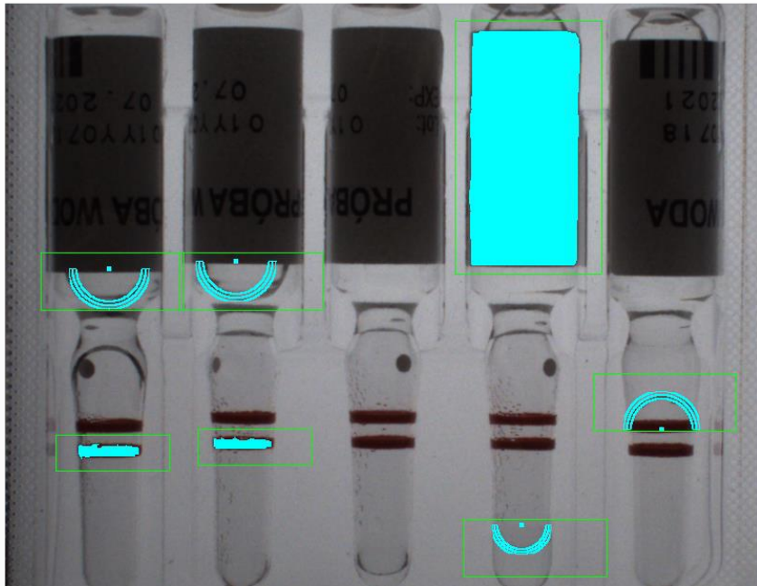
Liquid presence, label presence and ampoules ring check
