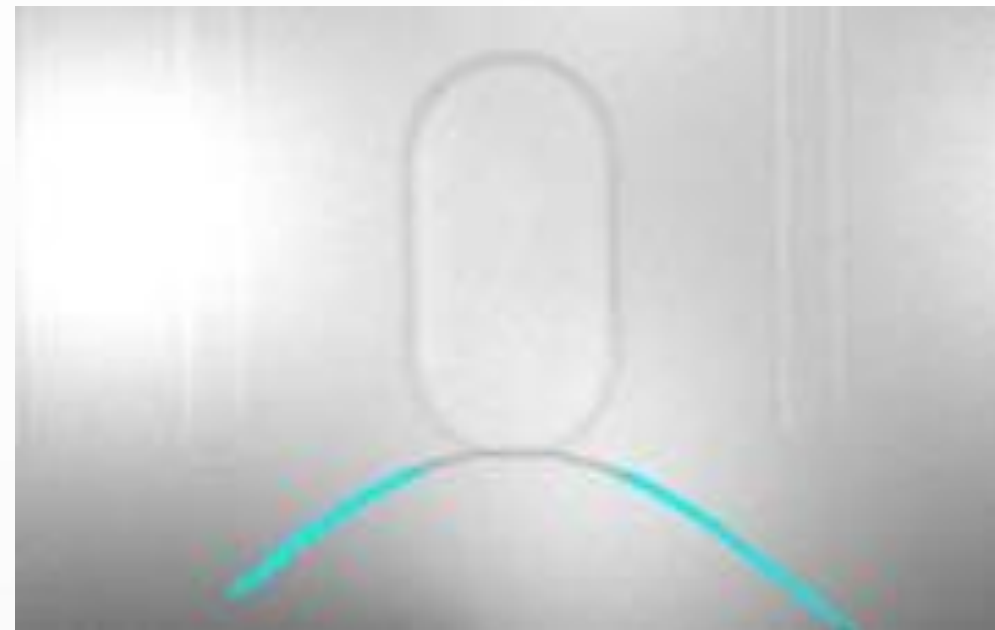
Presence of impurity and defect on the blister surface
