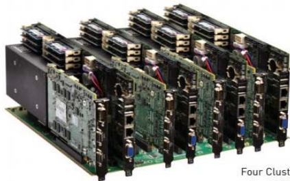
Four Clusters with: - One FPGA (Matrox Radiant eCL) - Two CPUs (Matrox SHB-5520)
