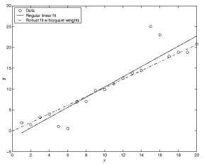
▶ the least square based methods are very sensitive to outliers due to the quadratic error function  $\rho(r_i) = r_i^2$
