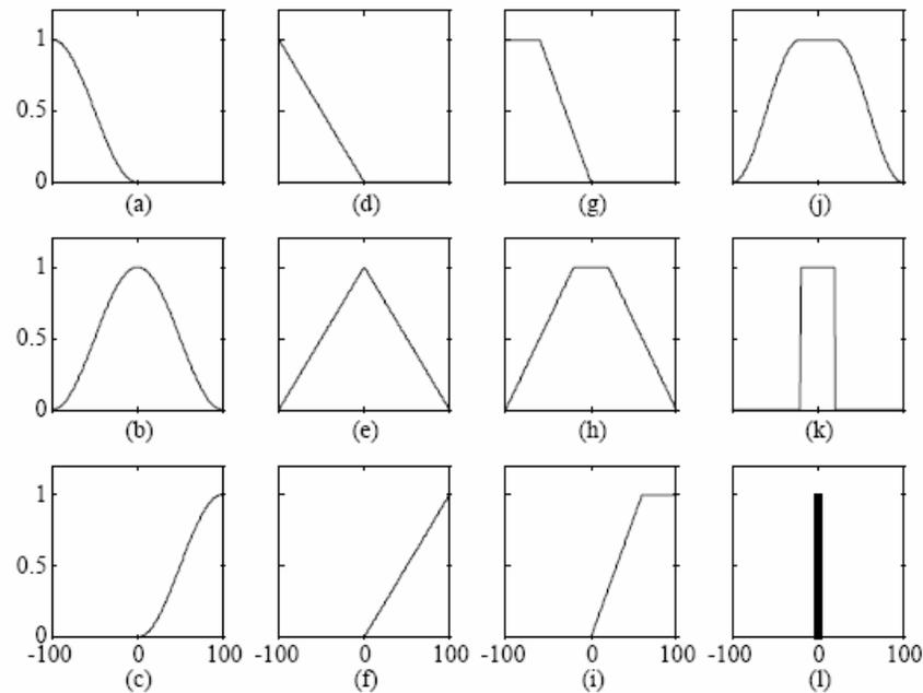
Figure 6: Examples of membership functions. Read from top to bottom, left to right: (a) z-function, (b)  $\pi$ -function, (c) s-function, (d-f) triangular versions, (g-i) trapezoidal versions, (j) flat  $\pi$ -function, (k) rectangle, (l) singleton.
