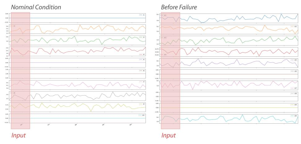
Training and Prediction occurs by using a sliding window of sensor readings as input
