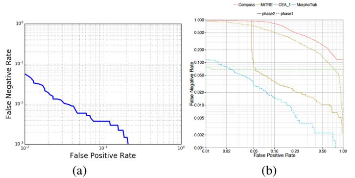
Fig. 2. The detection error trade-off (DET) plot between False Positive Rate (FPR) and False Negative Rate (FNR). (a) The proposed TATT-RBDL method. (b) Four algorithms reported in [7]. The blue curve in (a) consistently has lower FNR at the same FPR than all the curves in (b).
