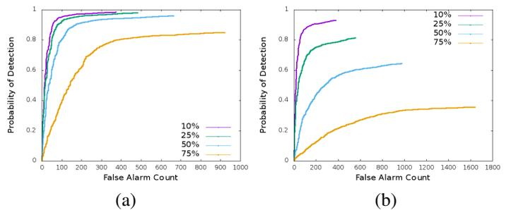
Fig. 3. Tattoo localization ROC between 2435 detection boxes and 2217 groundtruth boxes on Tatt-C dataset. (a) A true detection is counted when the overlap pixels between the boxes are at least 10% (purple), 25% (green), 50% (cyan), and 75% (yellow) of the pixels in groundtruth box. (b) A tighter condition when the overlap is at least certain percentage of both the groundtruth box and the detection box.
