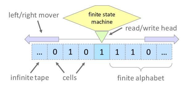
Assume that the tape is infinite and plenty of blank symbols o What does this machine do?
