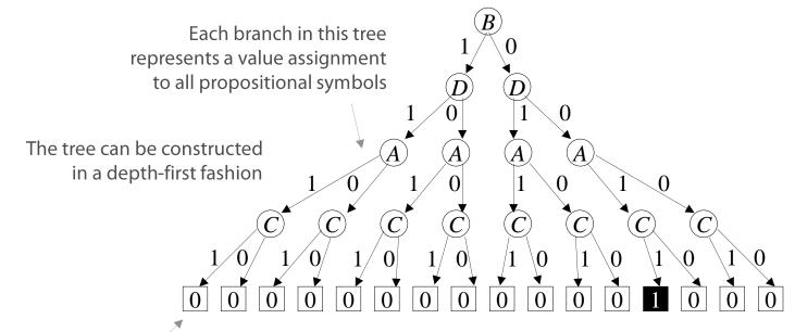
Each leaf in the tree is the value of the wff with the corresponding value assignments
