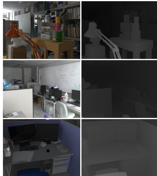
Figure 1: The new Tsukuba CG Stereo Dataset. A few example frames shown with ground-truth disparity maps among four sequences of 1800 stereo image pairs.
