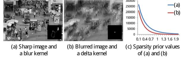
Figure 1. The x and y axes of (c) represent different  $\alpha$  and sparsity prior values, respectively. While both (a) and (b) produce the exactly same blurred image, the sharp image has higher sparsity prior values for all  $\alpha$ .
