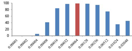
Figure 5. Percentages of images in Sun et al.’s dataset [19] satisfying  $f^{\text{IRLS}}(k_{gt})/f^{\text{opt}}(k_\delta) < 1$  with different  $\lambda_l$ .  $\lambda_l = 0.00064$  is the most effective to distinguish sharp and the no-blur solutions.
