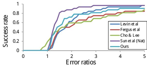
Figure 8. Performance comparison with Levin et al. [11], Fergus et al. [4], Cho & Lee [3], and Sun et al. [19] using the cumulative error ratio histogram proposed by [11] and Levin et al.’s dataset [11]. Success rates of other methods are from [19].
