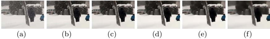
Fig. 3. ARF based image denoising. From left to right: (a) input, and denoised image using (b) \sigma = 10 , (c) \sigma = 15 , (d) \sigma = 20 , (e) \sigma = 25 , and (f) \sigma = 50 , respectively.
