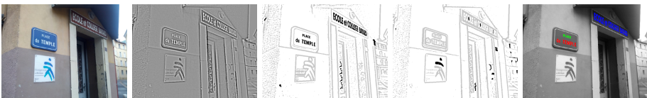
Fig. 2. Main steps of candidate text lines extraction: (from left to right) input frame, normalized contrast map, double binarization and filtering (retained components are shown in black), clustering into lines (blue, green, and red: three groups of components). Prudential criteria are used in filtering phases, in order to avoid the risk of discarding the text of interest.
