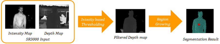
Fig. 1. Schema of the main steps of ToF based foreground segmentation. Input data are supplied by a SR3000, a modulated light ToF camera [2].
